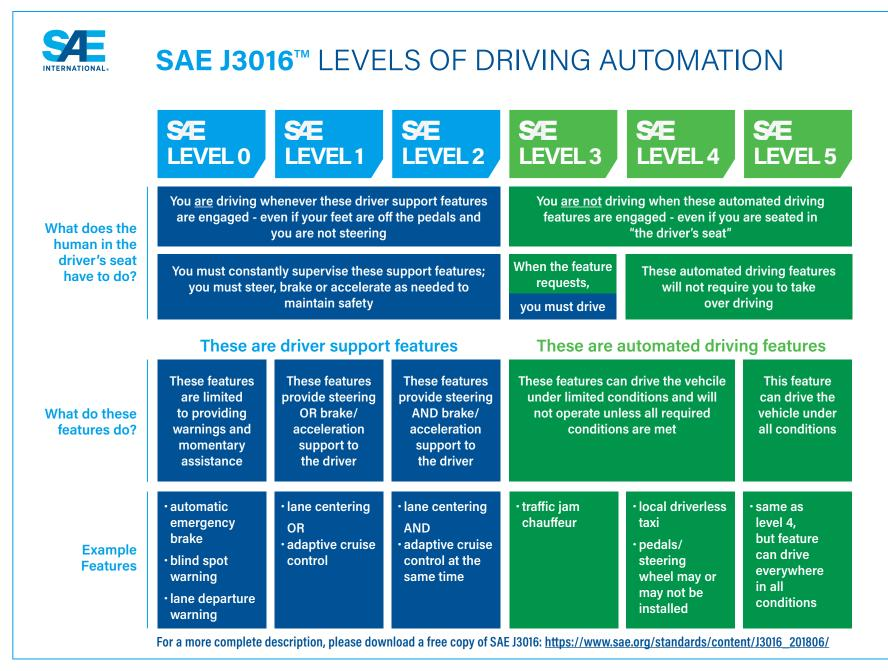
Figure 8: SAE Levels of Automation (www.sae.org)
